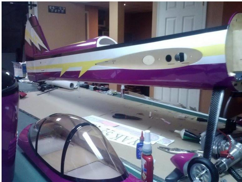
Next since I used a DA-50r and it has the same mounting pattern as a DLE-55 I went ahead and drilled the holes in the firewall.
