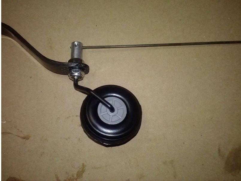
By this time the glue should have cured so you can at least work on the fuselage. I mounted my tailwheel and my main gear. To mount the main gear, I took a 1/4" socket and held the bolt with the screwdriver while tightening with the socket set.
