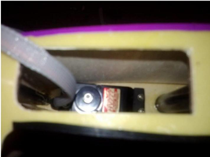
Next I went back to doing some gluing and I glued in the control horn pieces. I really like that the horns are colored. I also like the fact that the horn slots are precut and slotted. All I did was rough up the horns with sandpaper and then glued them in with 30 minute epoxy.
