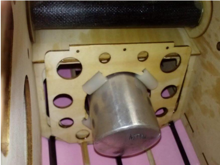
I went on and mounted my motor next. I used high temp red Loctite on the standoff bolts on both sides to assure nothing will come loose.
